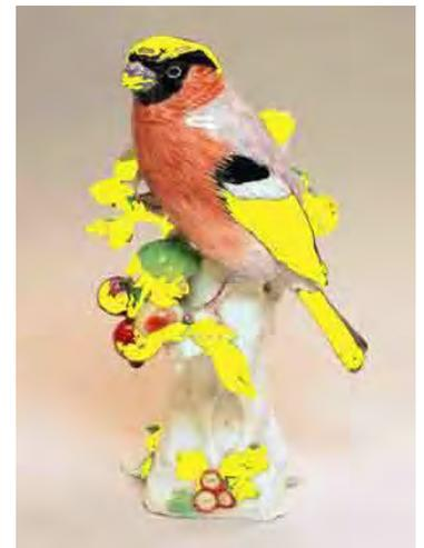
The two images are of the same bird. The yellow areas on the lower bird indicate the areas of 'invisible' restoration. The blue spectra is of an original glazed ceramic leaf, whilst the red spectra represents an over-painted / restored leaf.
